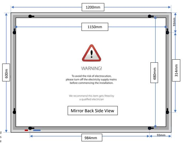
1. This product is IP44 rated so can be safety fitted in Zones 2 and 3. Position the mirror in a suitable location with at least 15cm clearance between the proximity sensor and the nearest surface and according to the zonal diagram show below, ensuring that the domestic electrical mains supply is within reach of the electrical entry point of the product.
