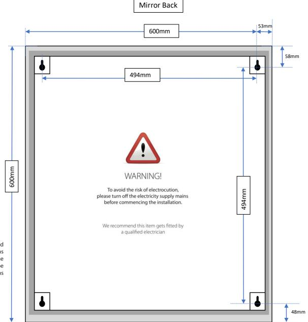
1. This product is IP44 rated so can be safety fitted in Zones 2 and 3. Position the mirror in a suitable location with at least 15cm clearance between the proximity sensor and the nearest surface and according to the zonal diagram show below, ensuring that the domestic electrical mains supply is within reach of the electrical entry point of the product.
