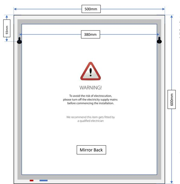
1. This product is IP44 rated so can be safety fitted in Zones 2 and 3. Position the mirror in a suitable location with at least 15cm clearance between the proximity sensor and the nearest surface and according to the zonal diagram show below, ensuring that the domestic electrical mains supply is within reach of the electrical entry point of the product.
