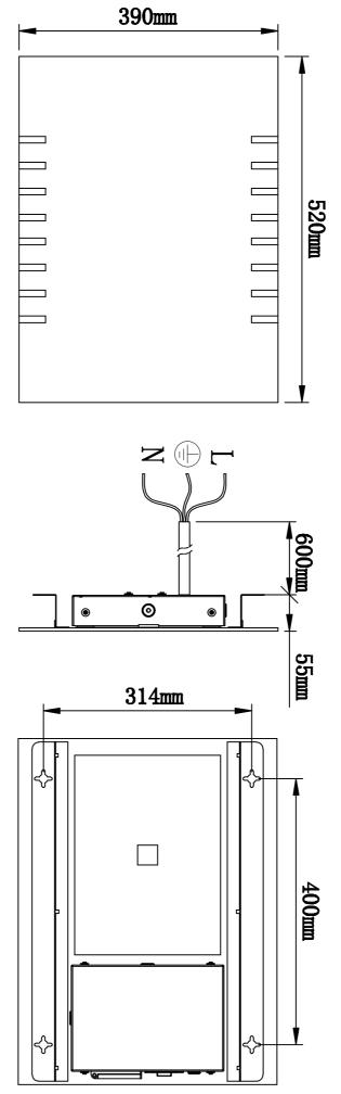
Remarks: The fixing sizes are same as the horizontal mirror (10011), but one is horizontal installation, another is vertical installation
