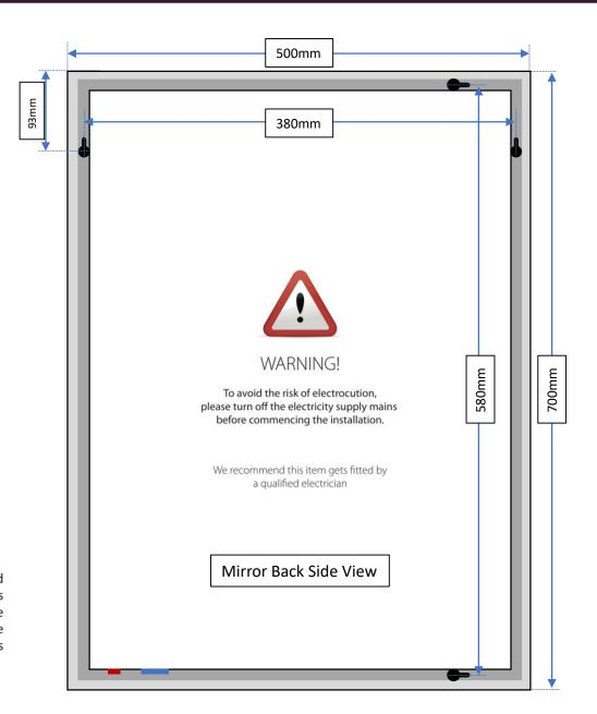
1. This product is IP44 rated so can be safety fitted in Zones 2 and 3. Position the mirror in a suitable location with at least 15cm clearance between the proximity sensor and the nearest surface and according to the zonal diagram show below, ensuring that the domestic electrical mains supply is within reach of the electrical entry point of the product.
