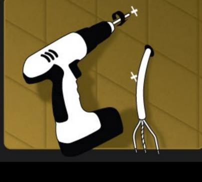
HAMMER WALL PLUGS INTO DRILLED HOLES AND SCREW THE 4 SCREWS INTO THE WALL PLUGS WITH PHILLIPS SCREW DRIVER.
